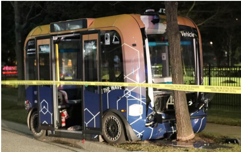
Figure 5-B: A Local Motors Olli vehicle after an accident that left the safety operator critically injured although it occurred at very low speed
