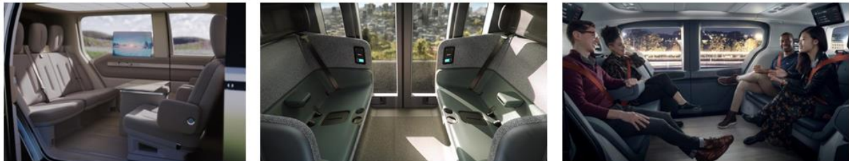
Figure 4-D: Seating layouts featuring rearward facing front row seats in Zeekr M-Vision (left), Zoox (middle), and Cruise Origin (right)
